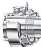
Figure 6. HMV nut and special stop nut for driving in a withdrawal sleeve.
